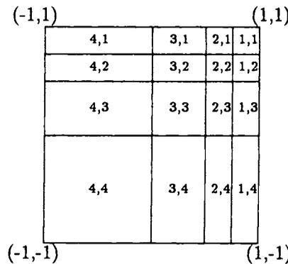
FIG. 1. Geometric mesh with polynomial degrees.
