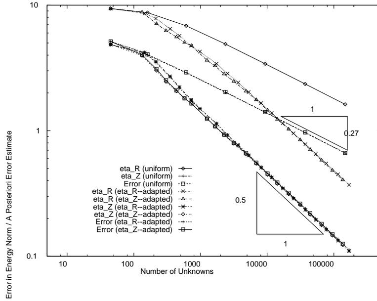
FIGURE 4. Errors  $e_N$  vs  $N$  for uniform and adaptive meshes of Example 6.1.
