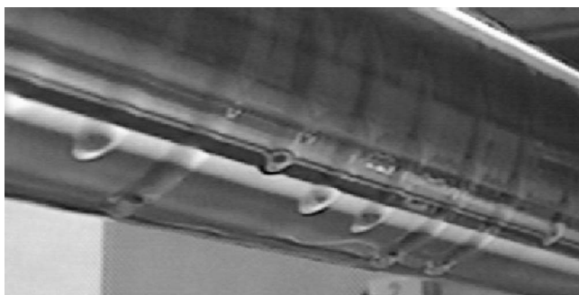
FIG. 23. Over time the droplets in the experiment shown in Fig. 20 accumulate the liquid and grow to form long fingers. The cylinder is seen from below the horizontal, and to one side.
