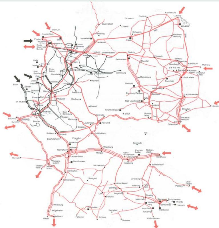
Figure 1.4. German H-gas (red) and L-gas (black) network systems. The arrows indicate entry and exit nodes. Gas storages are represented by black squares. (Source: OGE.)
