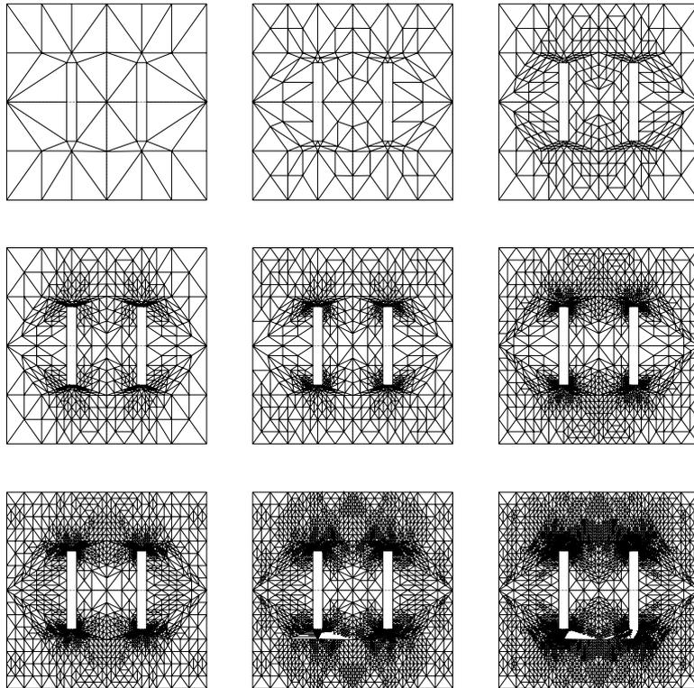
FIG. 5. Sequence of meshes  $\mathcal{T}_k$ , ( $k = 1, \dots, 9$ ) generated by Algorithm 1.
