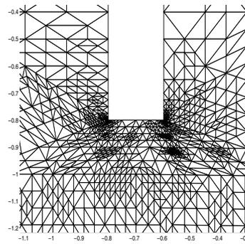
FIG. 4. Zoom view of the mesh near an inner corner of Fig. 3.
