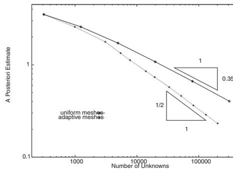
FIG. 6. Error estimates  $\eta_N$  for uniform and adapted meshes versus degrees of freedom  $N$ .
