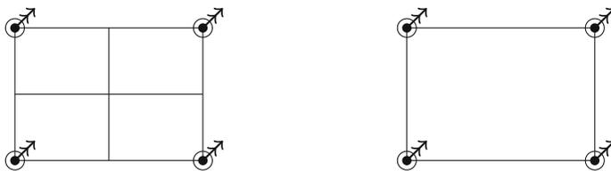
**Fig. 3** The  $C^1 - Q_2$  macro element and the BFS  $Q_3$  finite element
